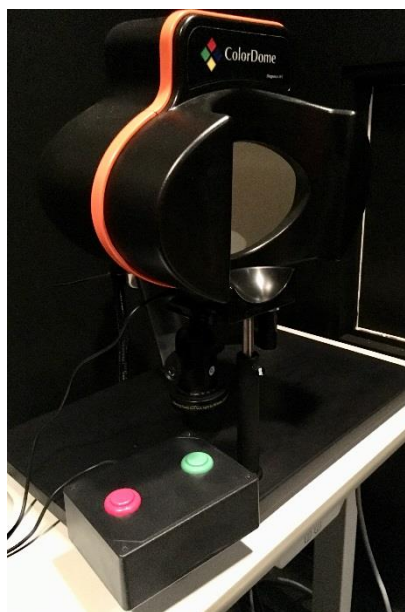
Figure 7. FST button box with ERG dome. Patients are required to indicate if they can perceive a flash of light while they are looking into the dome.
